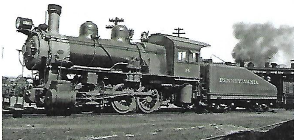
PRR 34 class B-8 0-6-0 Switcher, typical steamer of the CSLRR in the early 20th Century, supplanted by B-6sb.
